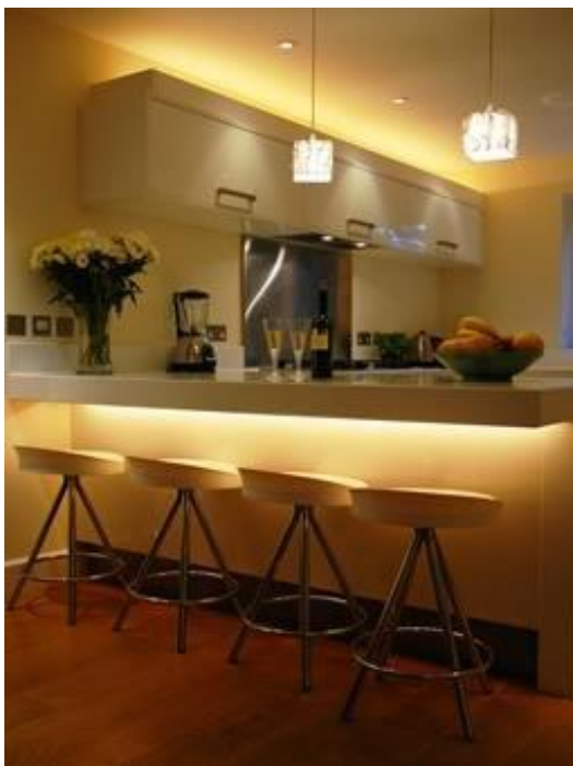
Cove Lighting and Under Cabinet Lighting
